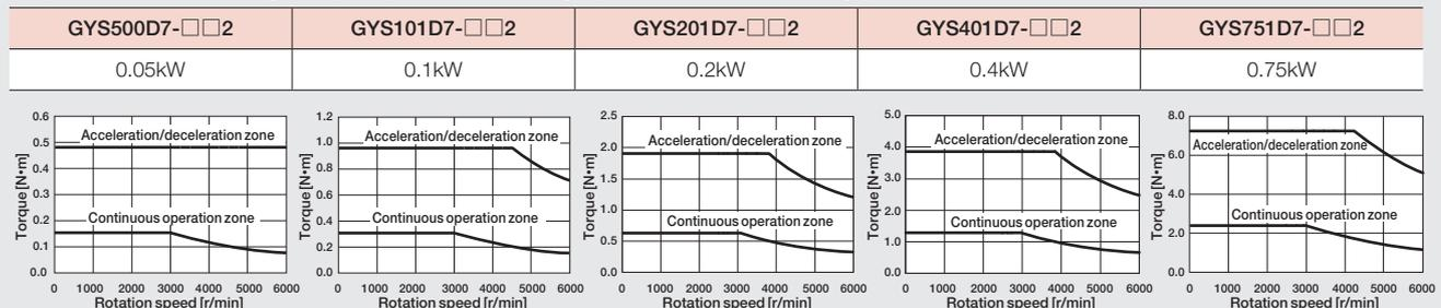
These characteristics indicate typical values of each servomotor combined with the corresponding RYT-7 type servo amplifier.
