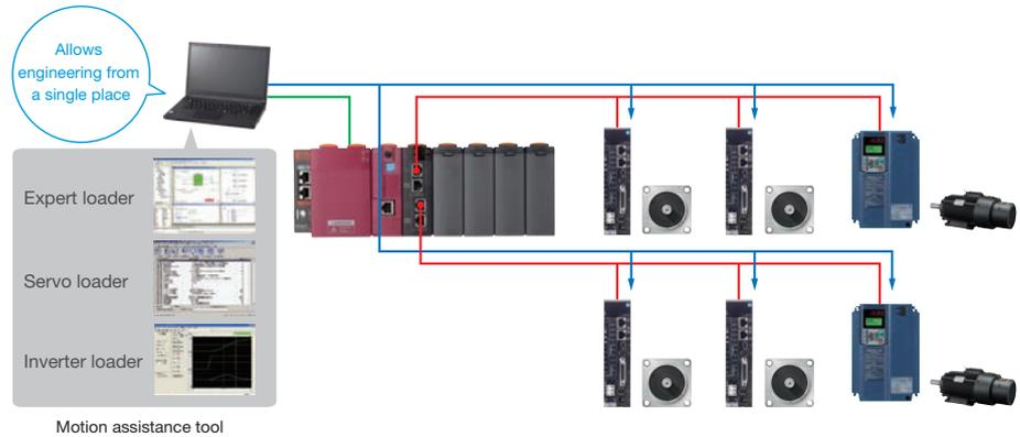
A single CPU performs both sequence and motion control
