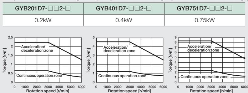
These characteristics indicate typical values of each servomotor combined with the corresponding RYT-7 type servo amplifier.
