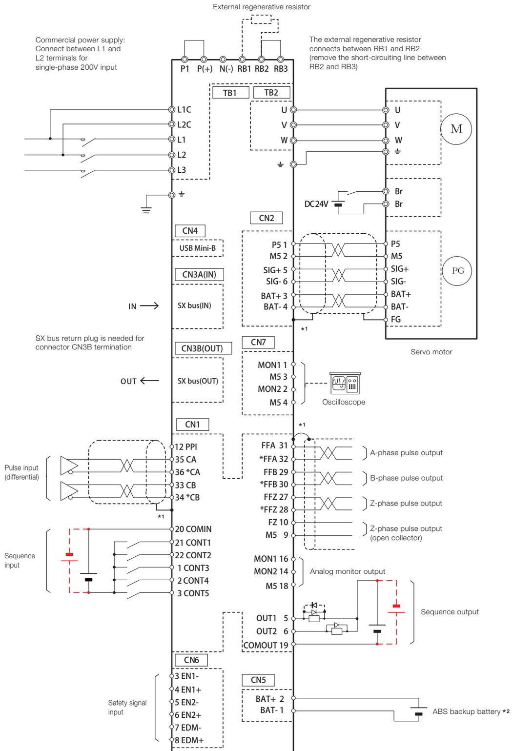
\*1: The shielded wire on the servo amplifier side connects to the connector shell.
