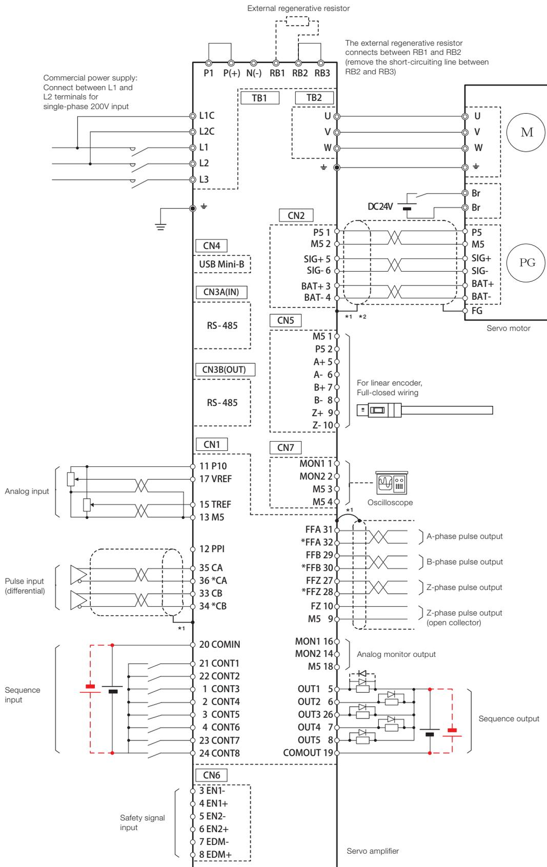
\*1: The shielded wire on the servo amplifier side connects to the connector shell.
