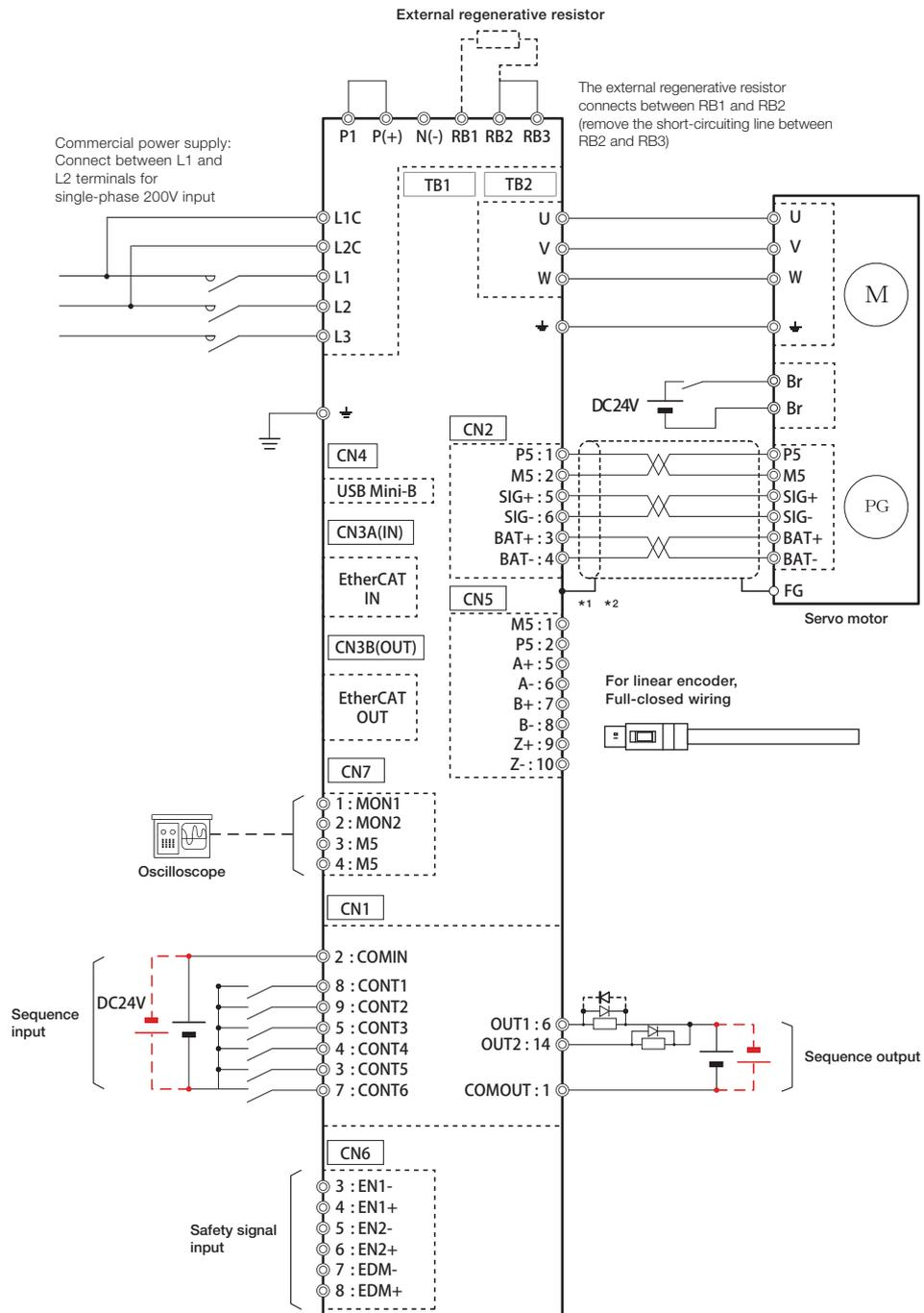
\*1: The shielded wire on the servo amplifier side connects to the connector shell.
