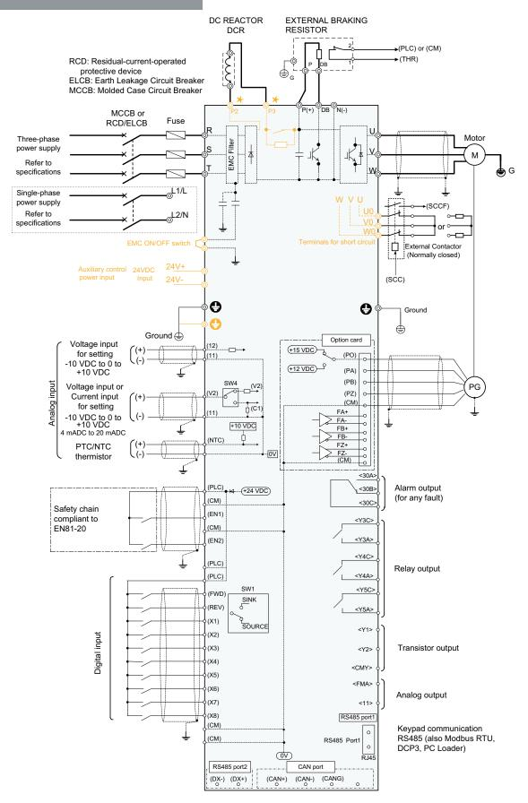
The orange marked parts represent the model "book type" lift inverter (FRN0032LM2A-4E or lower).
