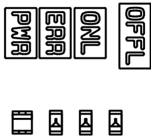
Figure 2.6 LED Status Indicators
