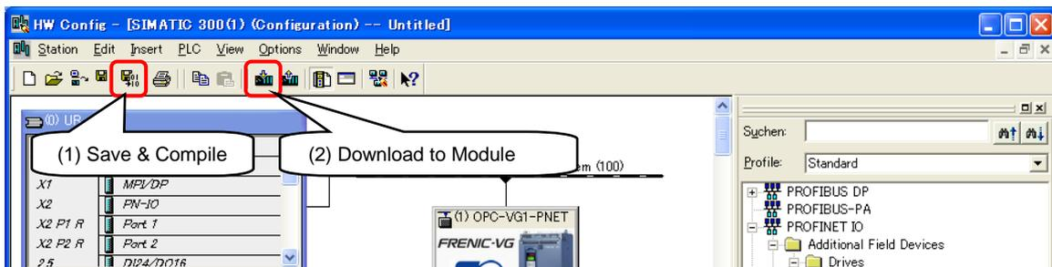
By far the configuration of PROFINET master device on STEP7 is finished.
