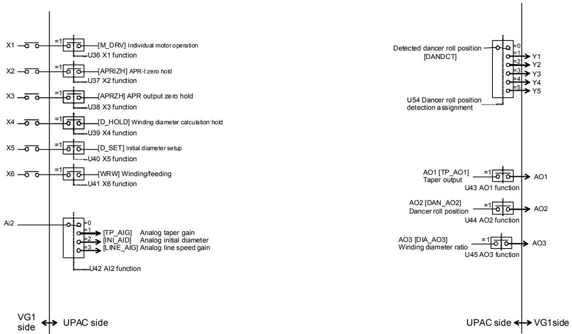
Fig. 4-1-3 Block diagram of UPAC dancer roll control software (3/4)
