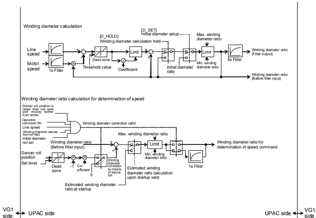
Fig. 4-1-3 Block diagram of UPAC dancer roll control software (4/4)
