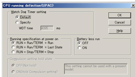
Fig. 1-3-41 CPU running definition dialog box
