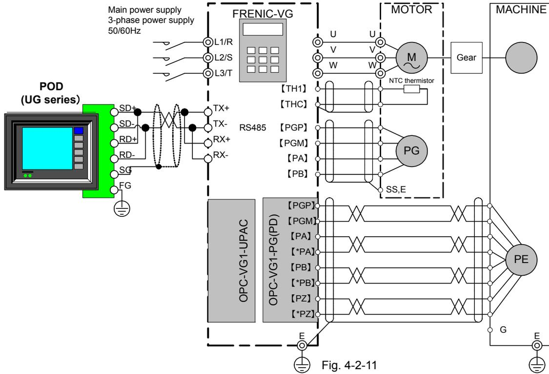
(4) Connection example using standard I/O terminal
