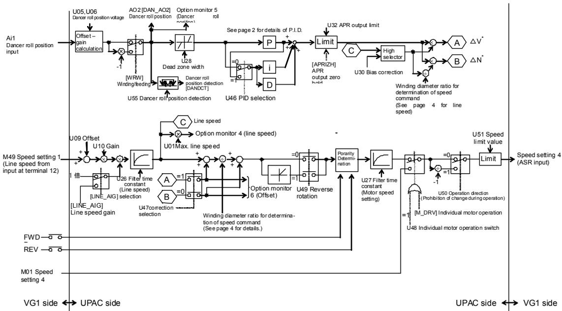
Fig. 4-1-3 Block diagram of UPAC dancer roll control software (1/4)
