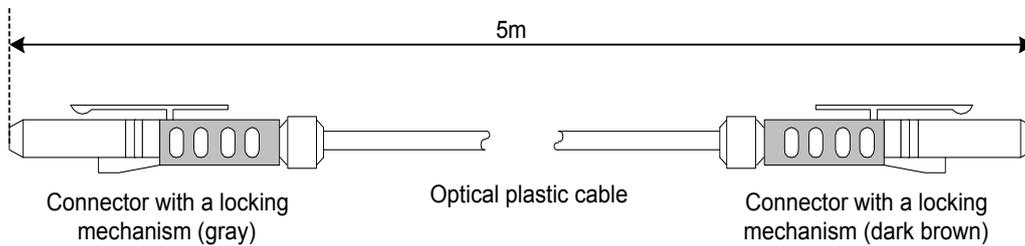
Fig. 1-2-5 Plastic optical fiber cable
