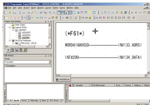
To reflect the change on FRENIC-VG, set the address (3Dh) of function code F61 and data (200d) on the worksheet.
