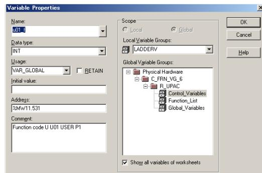
Select [OK] in the previous page to give the variable of u01\_f(UNO.01) to a worksheet as shown in the figure below.
