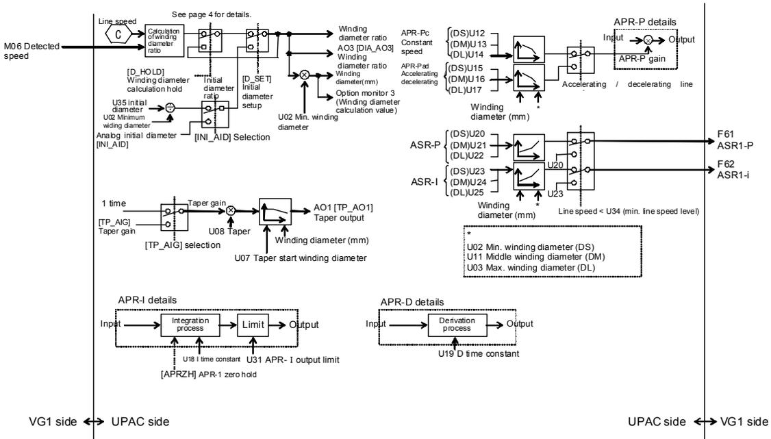
Fig. 4-1-3 Block diagram of UPAC dancer roll control software (2/4)
