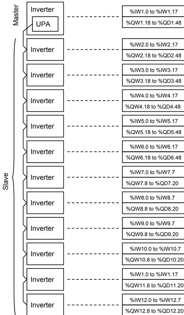
Figure 5-2-10 \* Input 8W and Output 14W (22W in total) are occupied for one inverter.
