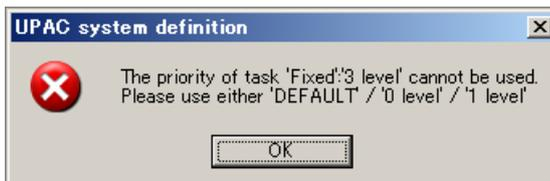
Fig. 1-3-44 Error message when you open system definition with invalid task settings
