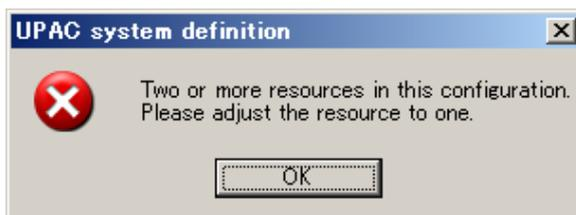
Fig. 1-3-42 Error message displayed when you open system definition with multiple resources
