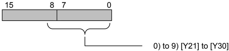
Compose the bits into word data before reflecting. An example of composition in the IL language is shown below.
