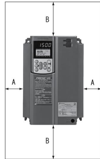
Figure 3.3-1 Mounting Direction and Required Clearances
