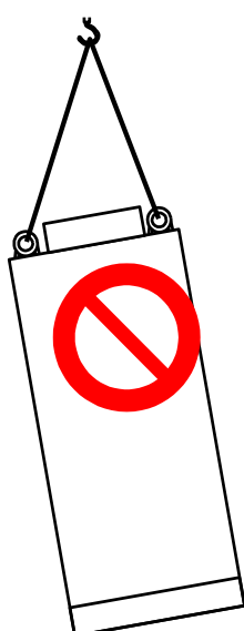
Figure 3.1-7: Tilt of cabinet (bad example)
