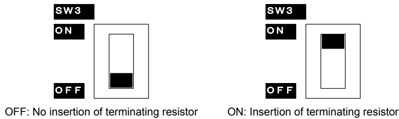
Figure 6.15.3 Terminating Resistor Switch Settings
